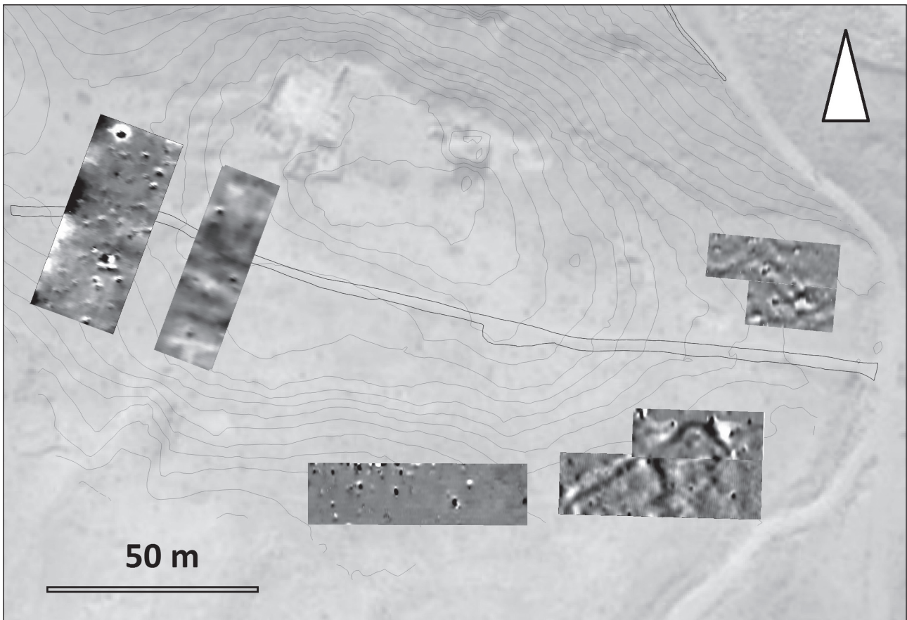
6. Magnetic gradient values show coherent linear anomalies, corresponding to walls in the easternmost areas (F. Berger).
